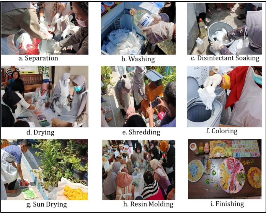
Fig. 2. Processing stages of baby diaper waste into resin handicraft products
