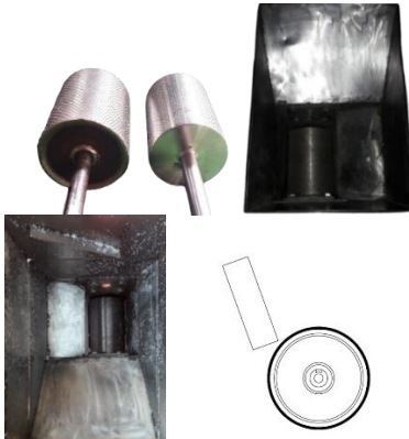
Fig. 2. Comparison of coconut grater designs showing the effect of teeth size and cylinder diameter on coconut meat residue
