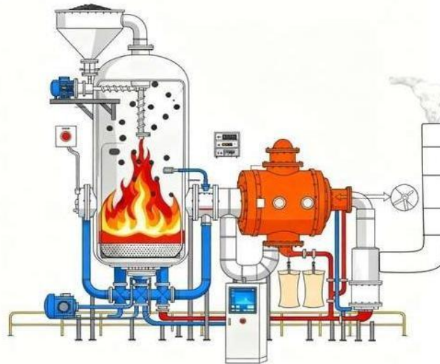
Fig. 1. RDF pellet reactor system with residual heat exchanger
