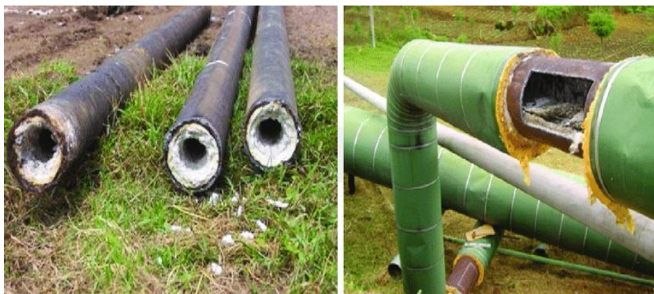
Fig 6. Amorphous Silica Scale on Re-injection Pipes (PT. Geodipa Energi, 2009)
