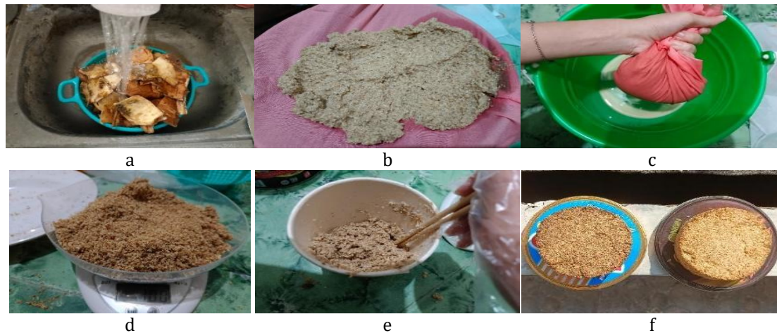
Fig. 1. Preparation of cassava peel samples: a) cleaning cassava; b) crushing cassava skin; c) pressing cassava skin; d) weighing cassava skin; e) mixing cassava skin with PVAc white glue; f) mixing cassava skin with PVAc white glue
