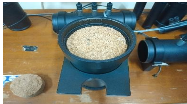
Fig. 2. Sample testing with the impedance tube method
