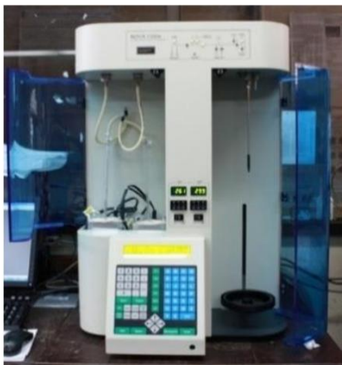
Fig. 6. Nitrogen Adsorption-Desorption Test Equipment with BET Method (Quantachrome NOVA 1200e Surface Area and Pore Size Analyzer)
