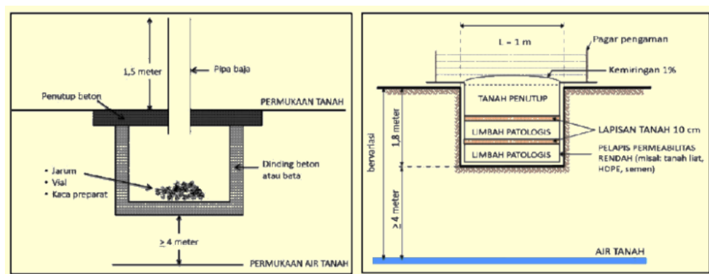
Figure 1. Construction of COVID-19 Hazardous Waste Burial
