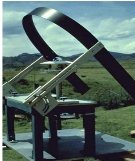
Figure 2. Shielded pyranometer for diffuse solar radiation
