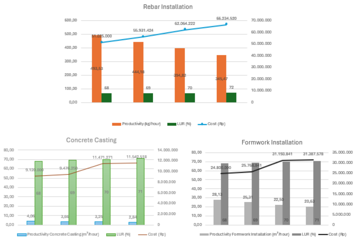
Fig. 3. Comparison of productivity, labour utilization rate (LUR), and cost across construction tasks under different overtime durations
