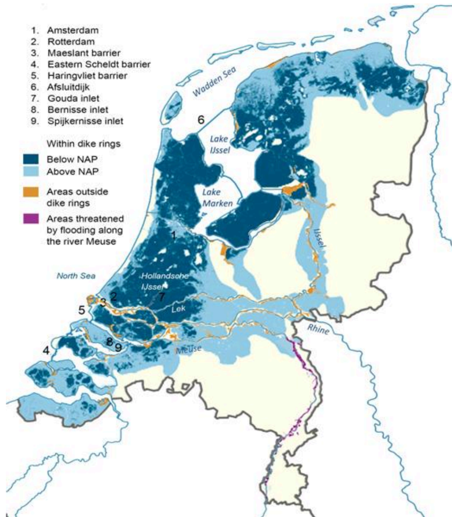
Fig. 2. Flood-prone zones in the Netherlands (blue shadings) and features of the water management system (Haasnoot et al., 2020)
