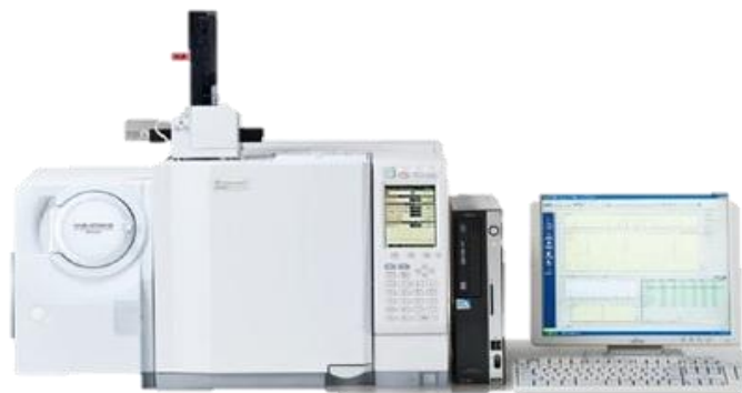
Fig 6. Gas chromatography – mass spectrometer (Gandjar & Rohman, 2007)
